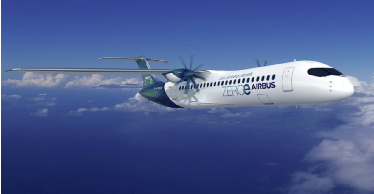
The AirbusZEROe turboprop concept, which would use liquid hydrogen fuel. (Credit: Airbus)
