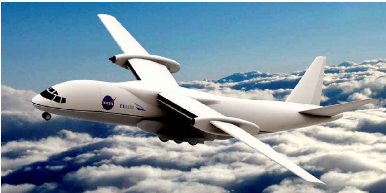
An example of a distributed electric propulsion design from Empirical Systems Aerospace (ESAero) for NASA. (Credit: ESAero)
