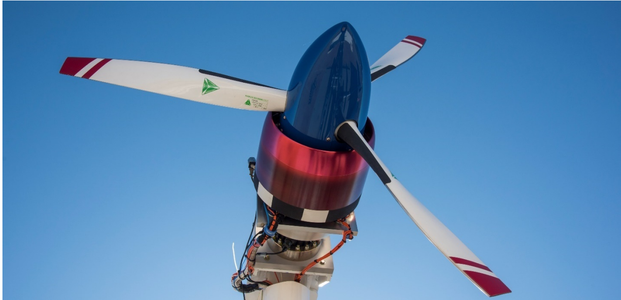
Electric engine with propeller seen on NASA's X-57 Maxwell's wingtip cruise motor/propeller. (Credit: NASA)
