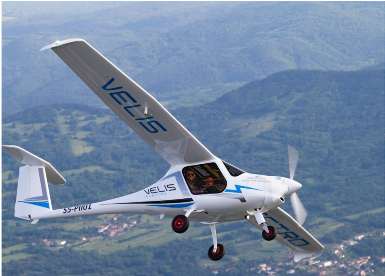
The Pipistrel Velis electric aircraft by the Slovenia-based company Pipistrel. The Velis is the first standard-type certified electric powered aeroplane approved for pilot training in Day VFR operations, having received certification in July 2020. The Velis is in serial production. (Credit: Pipistrel)
