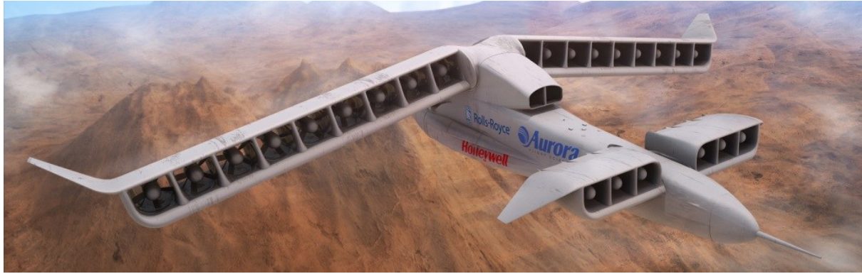
An example of distributed propulsion with the Aurora unmanned drone, which uses 24 distributed ducted fans and a tilt wing design. (Credit: Aurora)
