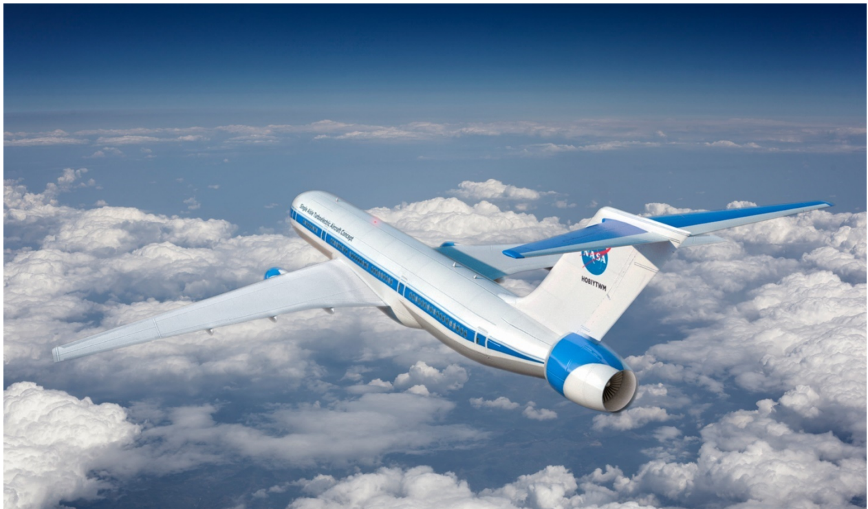
The NASA STARC-ABL, which stands for Single-Aisle Turboelectric Aircraft with Aft Boundary Layer propulsion. (Credit: NASA)
